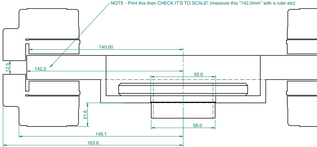
WMS 284mm Uno 4P007 profile - rotated COPYRIGHT/DESIGN RIGHT IN THIS DRAWING IS OWNED BY WORKS MOTORSPORT Email: keri@keri.co.uk Tel 07843 592 232
